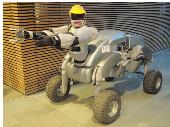
Fig. 1: Aalto University's WorkPartner robot is used as an astronaut-robot cooperation test platform.
