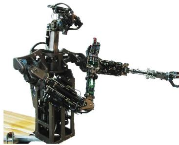
Figure 2.3: MIT's *Domo* robot, from Edsinger (2004).
