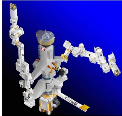
Figure 2.1: Special Purpose Dexterous Manipulator (SPDM) or *DEXTRE*, from Doetsch (2005).
