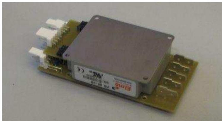
Figure B.1: Modified Elmo controller using custom made PCB
